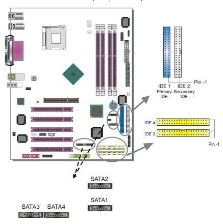
This Motherboard offers two primary (IDE1, IDE3) IDE device connectors, 2 secondary IDE device connectors (IDE2, IDE4) and 4 tertiary serial ATA ports. IDE1 and IDE2 can support up to four high-speed Ultra DMA 33/66/100 HDD or CD-ROM. IDE3 and IDE4 can support up to 4 high speed Ultra DMA 33/66/100/133 HDD. SATA1~4 can support up to 4 ATA 150 SATA hard disks.
